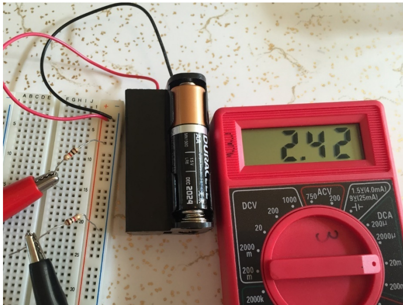
Figure 1.8: Circuit showing current measured with a Multimeter.
