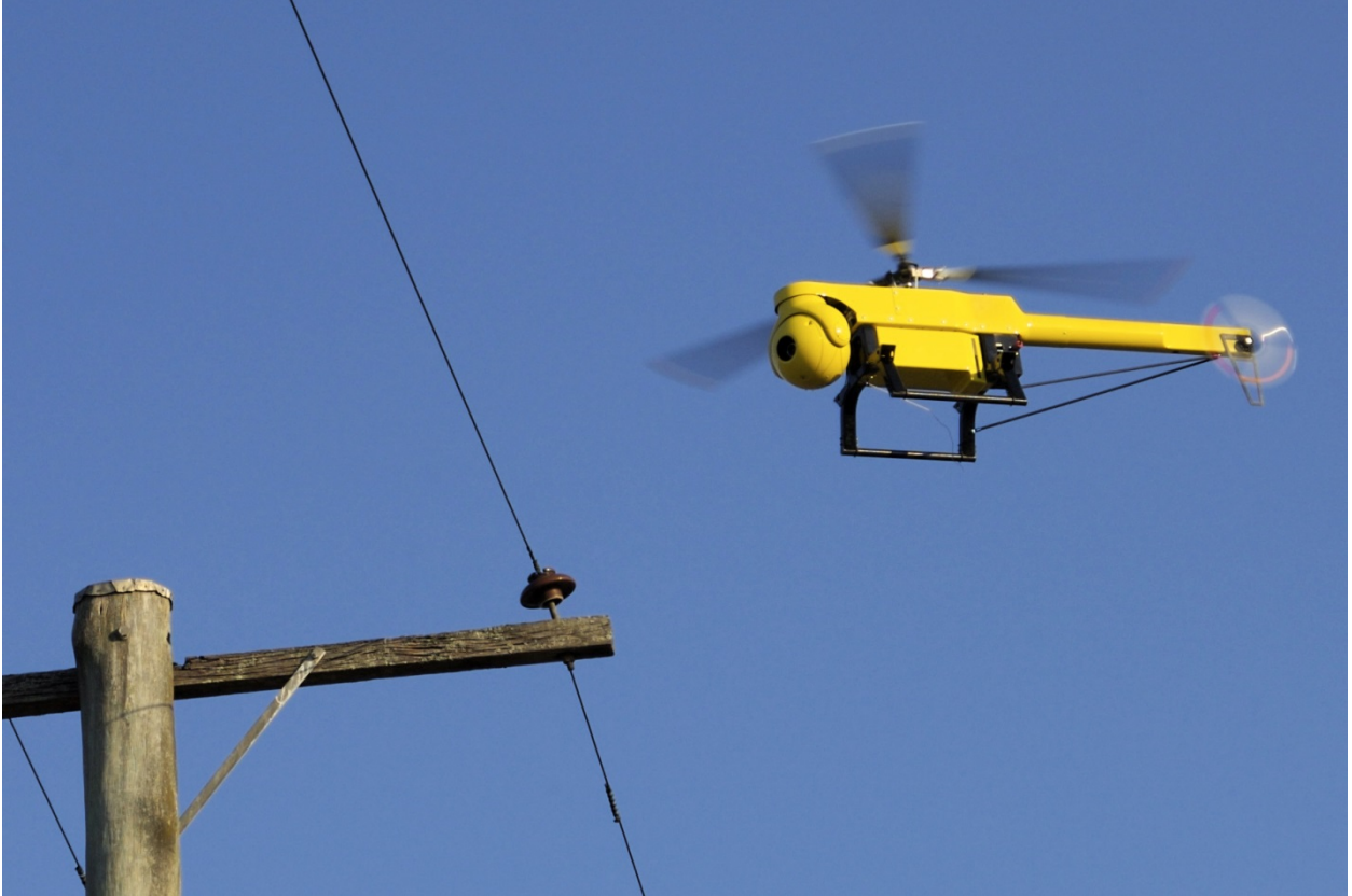
Figure 3.5 - An Unmanned Aerial Vehicle or 'Drone' used for Visual Inspection of Power Lines
