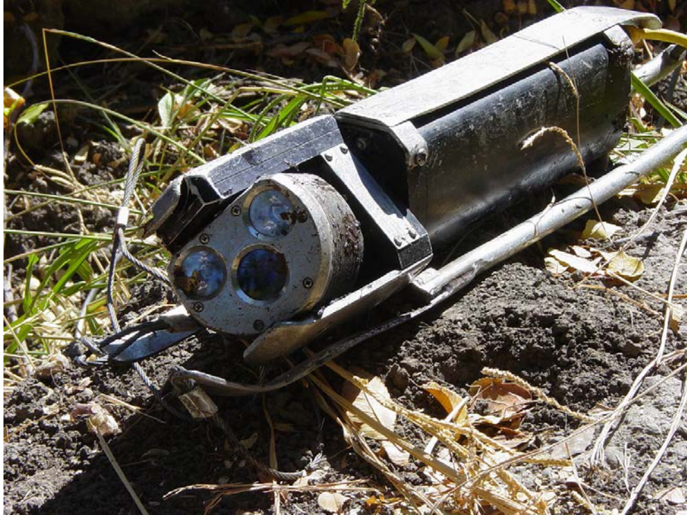
Figure 3.4 - A Video 'Pig' for Pipe Inspection
